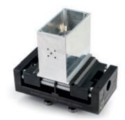
Example: 5-side machining with raw part clamping
